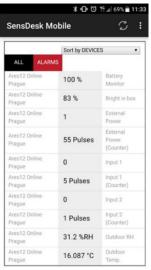
Portal function periodically sends the data to a remote server and the sending period is set by this server. AutoPush is a function allowing unusual measured data sending, beside the periodical logging, in case that the value change is higher than the AutoPush delta parameter.
